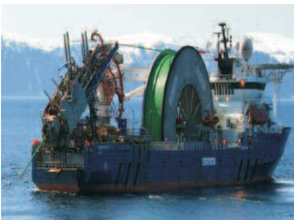
Reel barge used to lay CO 2 pipeline
