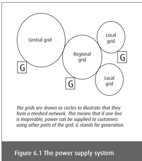
Figure 6.1 The power supply system
