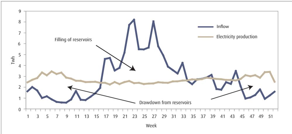
Figure 2.2 Variations in water inflow and electricity output in 2007.
