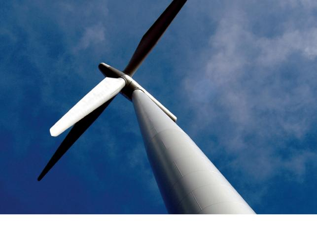
wing in motion provides lift to an aircraft. Energy is transmitted from the turbine via the propeller shaft to a generator inside the turbine head. The generator converts kinetic energy to electrical energy, which is then transmitted to transformers out on the network.
