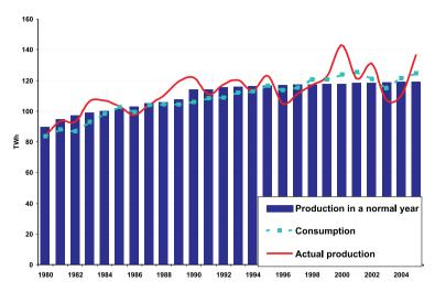
Figure 2.4 Trends in hydropower output and mean annual generating capability Source: Norwegian Water Resources and Energy Directorate
