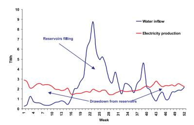
Figure 2.1 Variations in water inflow and electricity output during a year Source: Nord Pool
