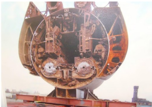
6. CUT SECTION IN TRANSPORT – N.B. KEEL CONSTRUCTION
