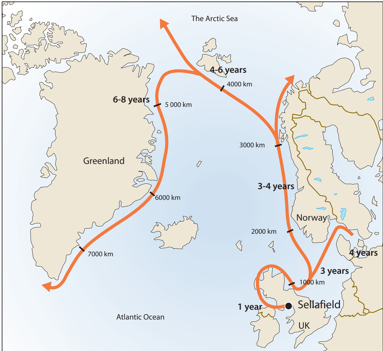
Figure 3.8 The map shows how caesium is carried from Sellafield by ocean currents. The route followed is the same as that followed by technetium. The map also shows how long it takes the caesium to reach the different areas once it has been discharged from the Sellafield facility.
