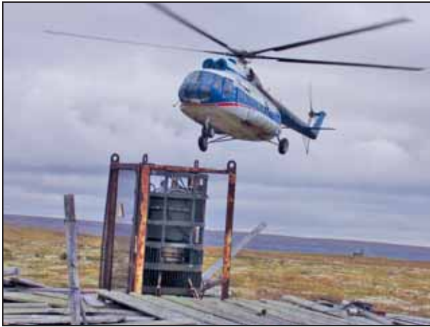
Figure 3.4 The RTGs have to be removed from inaccessible sites by helicopter.
