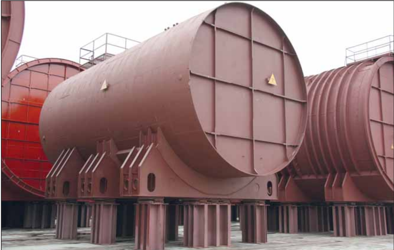
Figure 3.2 Reactor sections from nuclear submarines in storage at Saida Bay.
