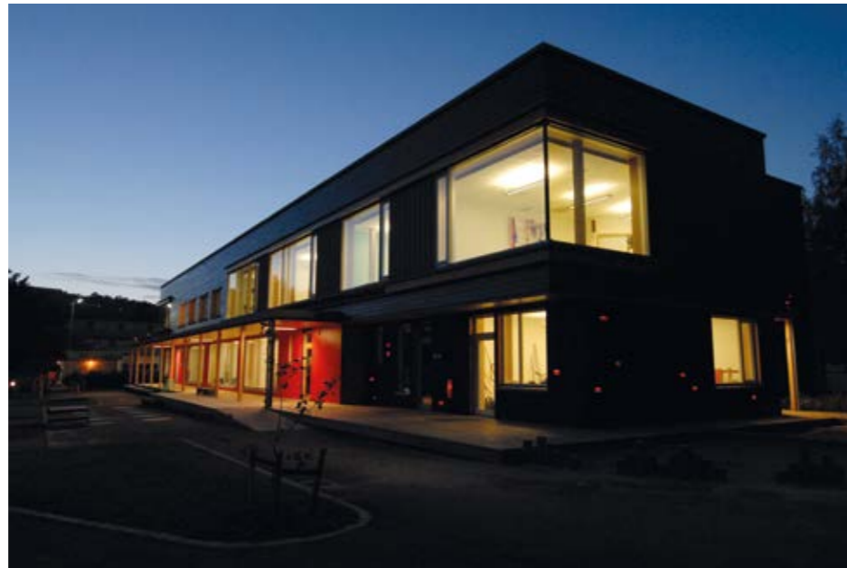
The entrance area with blocks that shine with different colours depending on whether the kindergarten is producing electricity or receiving electricity from the grid. Photo: Sidsel Jørgensen
