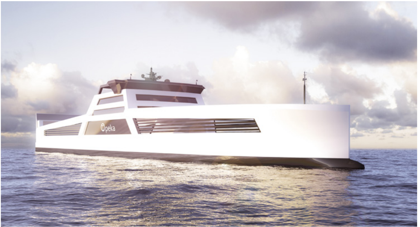
Topeka will be the world's first zero-emission hydrogen-powered cargo ship and will sail between Stavanger and Kristiansund. Illustration: Wilhelmssen and LMG Marin.
