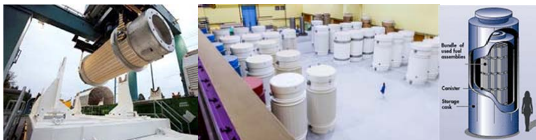
Figur 6-3 Ulike typer transportable lagringsbeholdere
